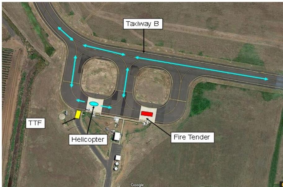
Figure 2: Layout for hot refuelling from bulk tankers
