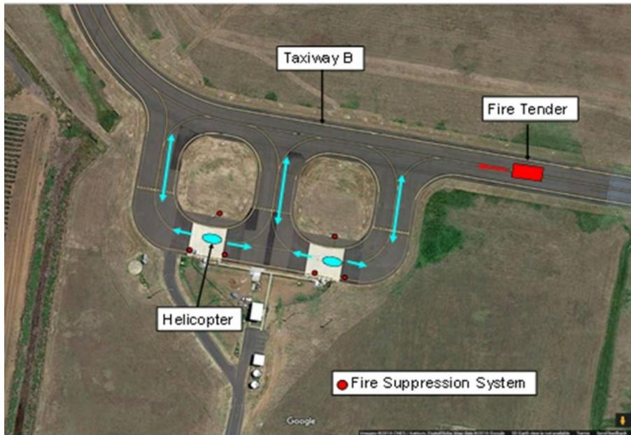
Figure 1: Simultaneous HREF Operations on two refuel pads
