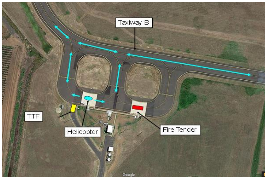
Figure 2: Layout for hot refuelling from bulk tankers
