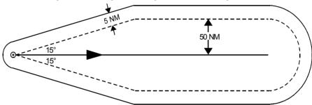
4.3.9 As for paragraph 3.5.2, but 10.3° lines expand to a maximum distance of 50NM either side of track. In no case is the maximum width of the basic area inside the 5NM buffer area greater than 50NM either side of track.
