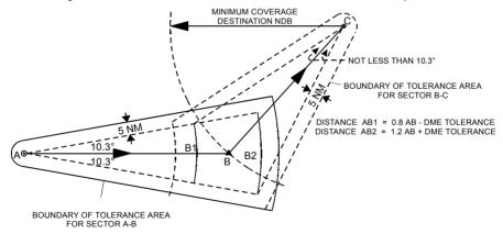
4.3.14 Route segment with change of direction at DME/azimuth aid fix. Coverage of destination navigation aid less than length of second sector of route segment.
