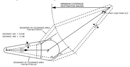
4.3.13 Route segment with change of direction at DME/azimuth aid fix. Coverage of destination navigation aid not less than length of second sector of route segment.
