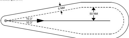
4.3.7 Route segment without navigation aids. Segment distance not exceeding 186NM (15° diverges 50NM from track in 186NM).
