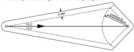
$4.3.3\,$  No navigation aid at departure aerodrome, destination navigation aid coverage such that  $10.3^{\circ}$  line intersect  $15^{\circ}$  lines from departure aerodrome.
