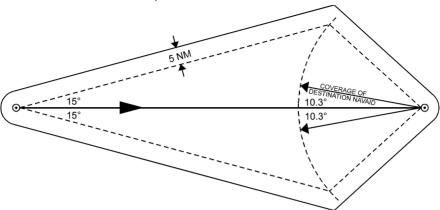
4.3.5 Navigation aid at departure aerodrome, no destination navigation aid. Segment distance not exceeding 275NM (10.3° diverges 50NM from nominal track in 275NM).
