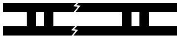
Figure 18(b) - New Additional Holding Position Marking Associated with Cat I, II or III Precision Approach Runways
