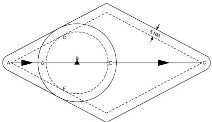
4.3.11 Route segments with change of direction at DR position. Coverage of destination navigation aid not less than length of second sector of route segment.
