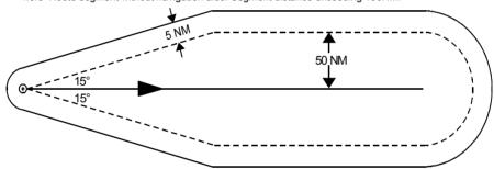
4.3.9 As for paragraph 3.5.2, but 10.3° lines expand to a maximum distance of 50NM either side of track. In no case is the maximum width of the basic area inside the 5NM buffer area greater than 50NM either side of track.
