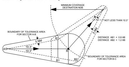
4.3.12 Route segment with change of direction at DR position. Coverage of destination navigation aid less than length of second sector of route segment.
