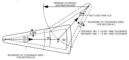
$4.3.14 \quad \hbox{Route segment with change of direction at DME/azimuth aid fix. Coverage of destination navigation aid less than length of second sector of route segment.}$
